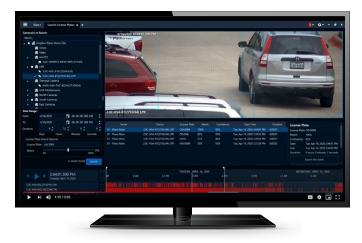
LPR analytics automatically read license plate information from vehicles, linking it to live and recorded video. This enables security operators to detect the presence of vehicles of interest in real-time or search, using full or partial numbers, and quickly find specific captured license plate video for further verification and investigation.
